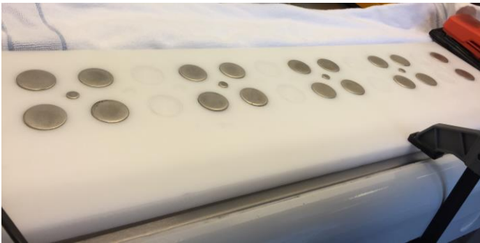
Figure 3. Nickel discs (large and small) to be ground in a specially produced disc holder.
