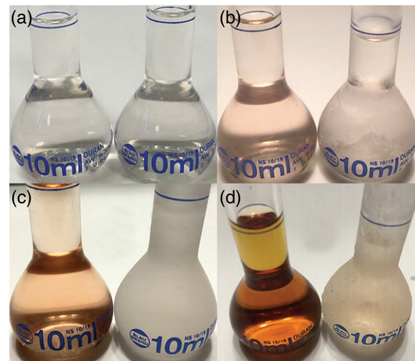
Fig. 3. Development of the diphenylcarbazide reagent over time under different conditions: the left glass beaker was stored at room temperature (22–23°C) without sunlight protection; the right glass beaker was stored at –18°C in darkness. (a) After 0 hr. (b) After 4 hr. (c) After 1 day. (d) After 60 days.
