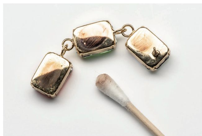
FIGURE 2 An inconclusive DMG spot test of an earring with known nickel (0.87 \mu\text{g}/\text{cm}^2/\text{week} ) and copper release (43 \mu\text{g}/\text{cm}^2/\text{week} ), due to a masking effect caused by brown discolouration of the DMG test reacting with released copper. DMG, dimethylglyoxime
