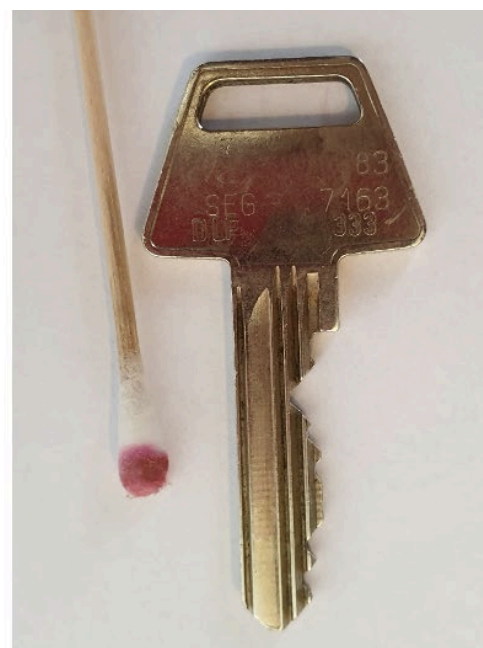
Figure 2. Left: chelation of nickel with two DMG molecules to form a nickel DMG-complex. Right: A positive DMG test shown by the bright red discoloration after the spot testing of a key.
